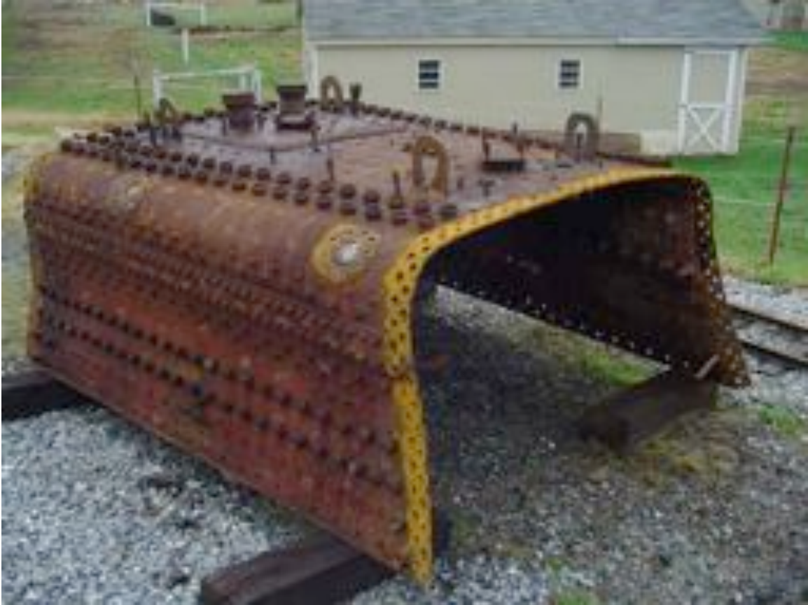
The old upper side sheets and roof sheet, removed from the firebox, rests outside at the Strasburg Railroad Company Erecting Shop.
